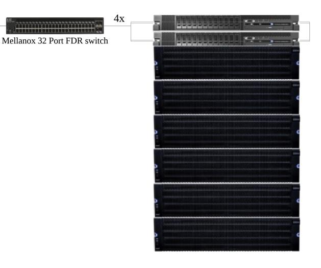
1 GSS24/26 depending on the test. 2 FDR Ports connected per Server GPFS 3.5.0.7 GA code level
