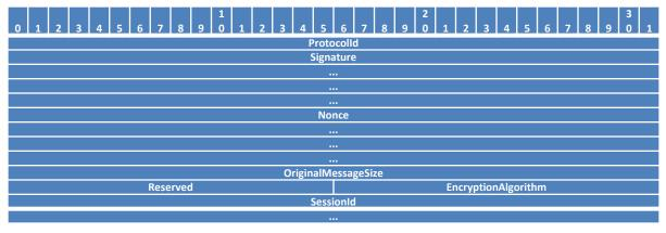
**EncryptionAlgorithm (2 bytes):** The algorithm used for encrypting the SMB2 message. This field MUST be set to one of the following values:
